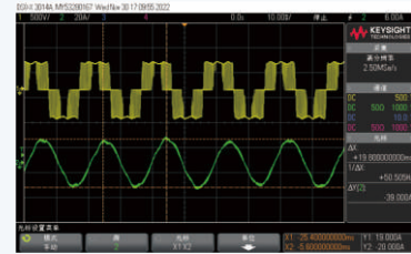
Current waveform under full load 50 Hz
